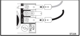
Fig. 41 Attach switch wires to valve.
